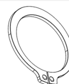
Shaft is used with elastic retaining ring Ø25
